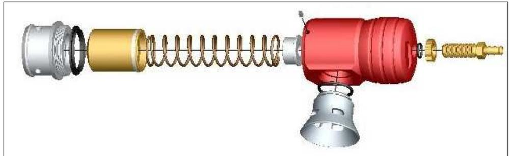
Wipe all internal parts clean with a rag. Inspect the piston and bore for visual damage, then slide the piston into the bore dry to check that it slides smoothly and freely. If any damage is found or the piston does not slide freely, contact GFB for advice. Otherwise, smear the piston and bore with engine oil and re-assemble.
